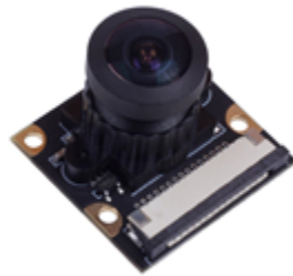
Figure 11: IMX219 Camera Sensor NVIDIA Jetson Nano [6].
