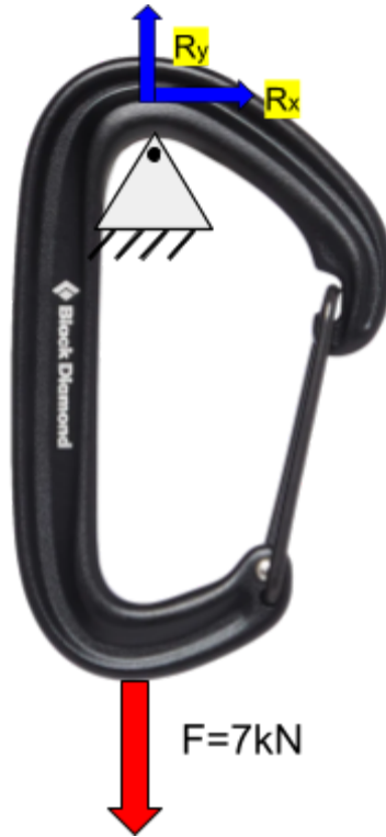
Figure 1: Carabiner illustrated with force load and fixed pin-support
