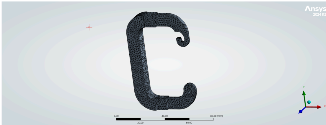
Figure 10: Updated model with mesh element set to 1.25 mm and resolution set to 6.
