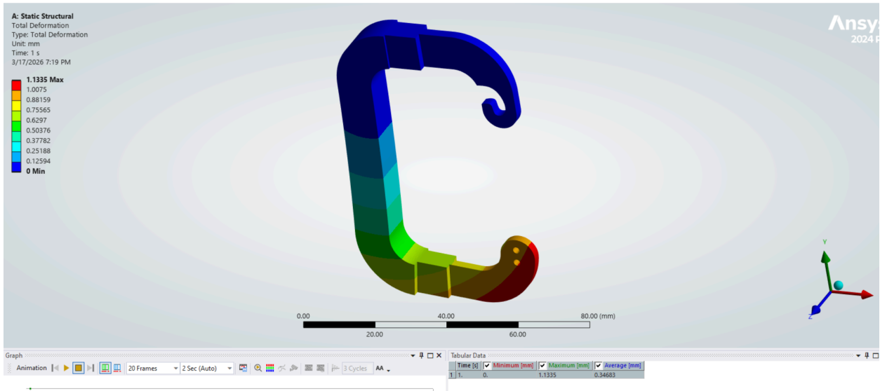
Figure 12: Updated model with maximum deflection of 1.1345mm.
